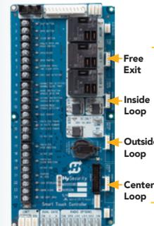
HY-5A Vehicle Detectors (up to 4) plug into sockets
