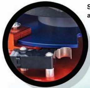
Simple limit switch arrangement
